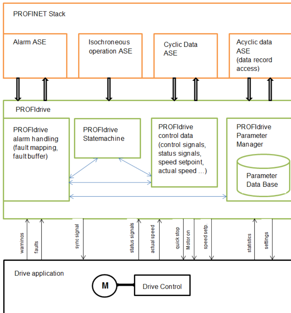
Figure 2-1 Overview: PROFIdrive (green) as the application layer between the PROFINET stack (orange) and the drive application (black) from drive perspective
