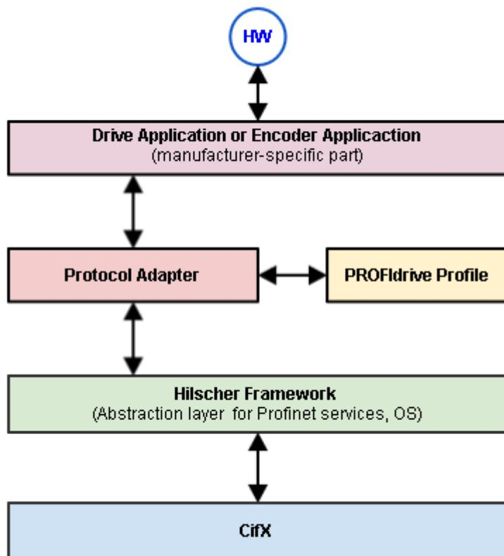
The complete configuration is divided into several subjects. Excepting Profidrive profile configuration, all configurations will be posed by the Application. These configurations will be listed either in Drive\_config.c or in Encoder\_Config.c depending on used application.
